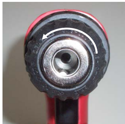
To Remove the Chuck Twist it Anticlockwise
