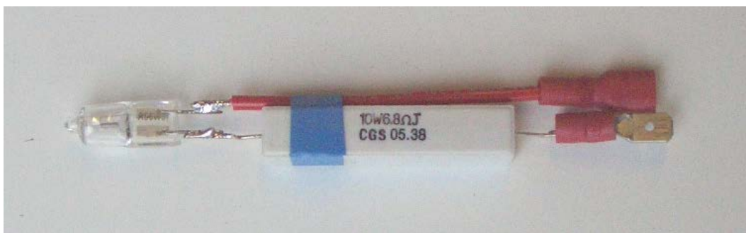
12v Halogen Bulb and 6R8 10W Resistor for Initial Testing of Small Motor
